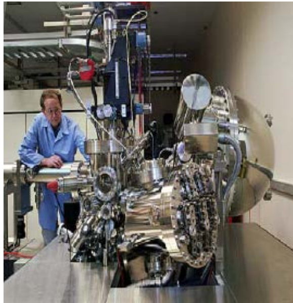
Fig. 43. MBE chamber (From the Internet).
