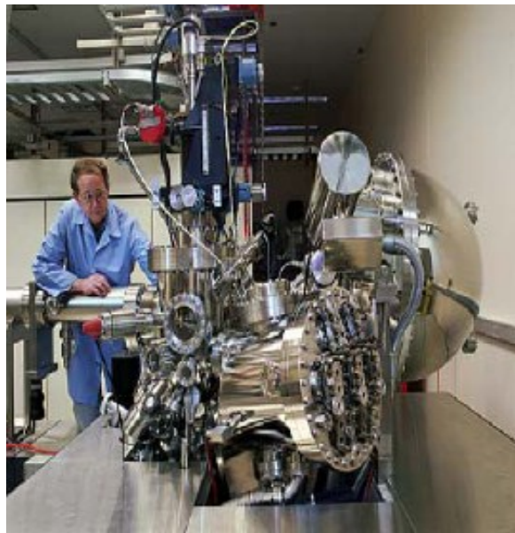
Fig.5.1 MBE chamber (From the Internet).
