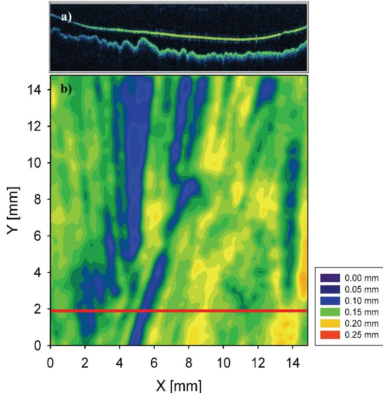
Fig. 5. (a) One of 200 OCT tomograms of the varnish layer over the fragment of oil paint; (b) a thickness map of the varnish layer obtained from a series of tomograms. The thickness is coded in false colours, red line indicates position of the tomogram shown in figure a
