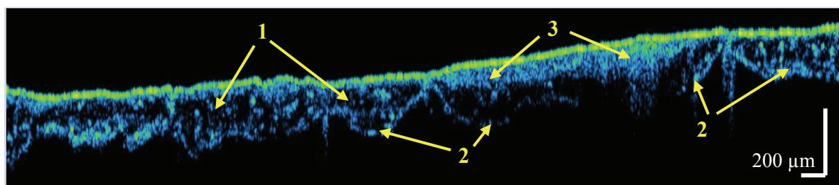
Fig. 4. Example of the inscription (arrow) located over the old paint layer: (1) varnish layer, (2) paint layer under varnish, (3) inscription painted over the original varnish-paint layer structure
