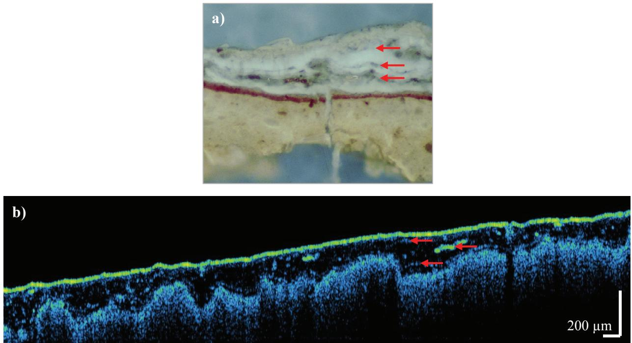
Fig. 3. Example of the multi-layered varnish over the paint layer: (a) microphotograph, UV excited fluorescence; (b) OCT tomogram. Arrows point to interfaces between consecutive varnish layers
