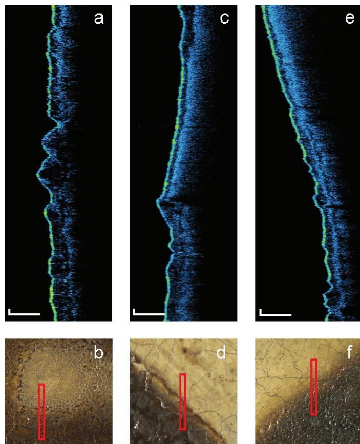
Fig. 2. (a) OCT tomogram from the Child's leg and its location (b); (c) OCT tomogram of the Child's hand and its location (d); (e) OCT tomogram of the Child's eyebrow and its location (f). Bars indicate 200 µm
