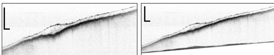
**Fig. 4.** The effect of refraction correction. (*Left*) an uncorrected image, bars indicate 0.2 mm in varnish ( $n = 1.5$ ). (*Right*) a corrected image, bars indicate 0.2 mm of geometrical distances. The picture examined was tilted to eliminate specular reflection from the varnish layer
