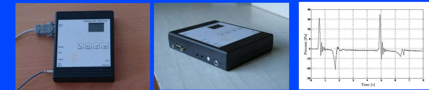
Perturbation of pressure in the room caused by opening the window (two times)
