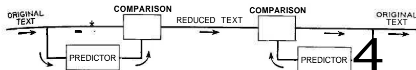
Fig. 2--Communication system using reduced text.
