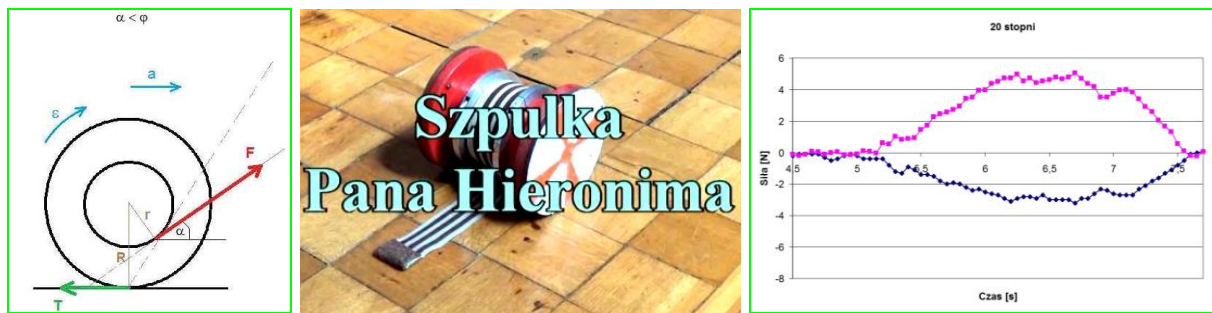
Fig. 2: From simplified picture of the situation in the Problem Collection (left panel) to a real demonstration (middle) and computer-aided experiment (right). The direction of movement of a rolling bobbin depends on the angle of the pulling force; the friction force is opposite to the pulling force, and is always in a constant ratio to it, depending on the angle. Adopted from ref. [7].
