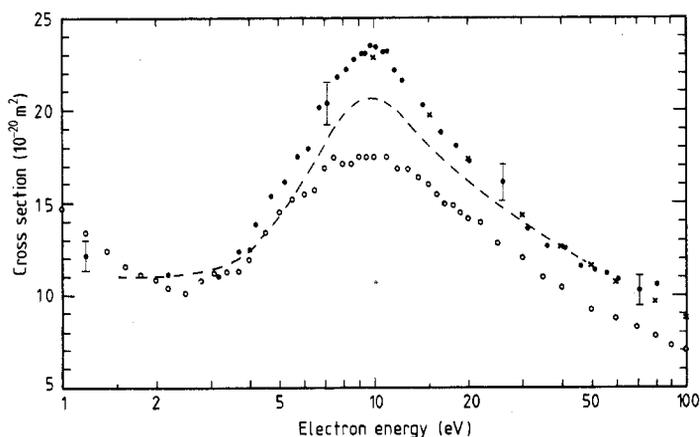
**Figure 1.** Total cross sections for electron-ammmonia scattering. Experiment: ●, present results, absolute; ---, Brüche (1929), absolute; ○, Sueoka *et al* (1987), normalised. Theory: +, Jain (1988). The error bars correspond to the overall experimental uncertainties at some selected points.
