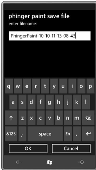
The only parts of this screen you can customize are the text strings in the headings and the initial text in the text-entry box. The screen looks much better in portrait mode than in landscape mode. In landscape mode, all the text headings, the text-entry box, and the on-screen keyboard are re-oriented but the two buttons are not, and the combination looks very peculiar. One look at it and you might never call *Guide.BeginShowKeyboardInput* from a landscape-mode program!
