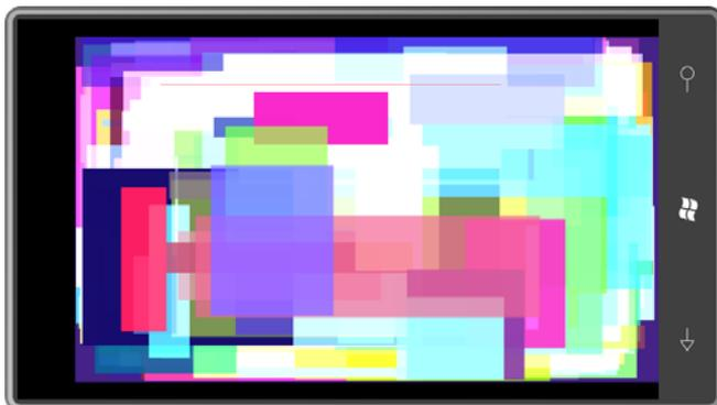
The colors used for the rectangles include a random alpha channel, so in general (as you can see) the rectangles are partially transparent. Interestingly enough, you can still get this transparency even if the rectangle being rendered has no alpha channel. Change the creation of *tinyTexture* to this:
