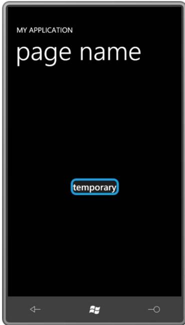
The button still displays the text “temporary” and it should really be displaying the text “Click me!” You might be tempted to put a *TextBlock* in there and set its *Text* property to a *TemplateBinding* of the *Content* property of the *Button*:
