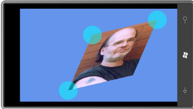
This program uses an affine transform, which means that rectangles are always mapped to parallelograms. The fourth corner isn't draggable because it's always determined by the other three:
