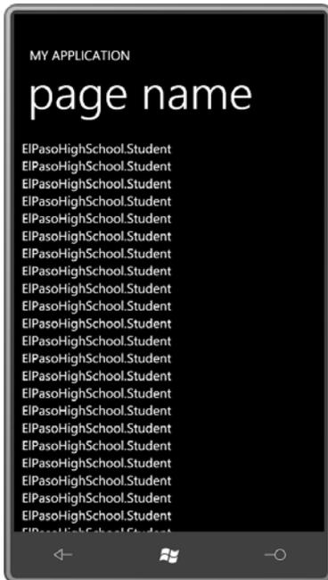
Whenever you see a *ListBox* or *ItemsControl* with a bunch of identical class names listed, don't despair. You should instead rejoice! Such a display shows that the *ListBox* has been successfully filled with items of the same type, and all it needs to display something meaningful is a *DataTemplate* or (if we're lazy) a *DisplayMemberPath* setting;
