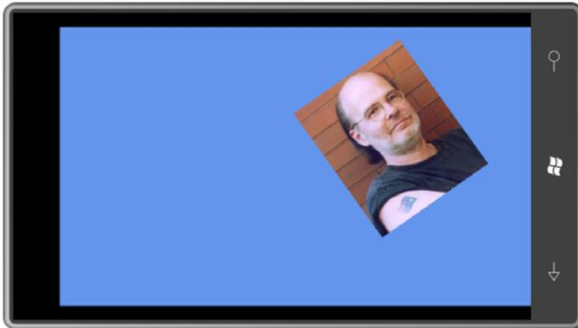
Of course, the most common form of scaling implemented in multi-touch applications involves two fingers in a pinching or stretching gesture, and in a sense, that isn't much more difficult than what you've already seen. I've been stretching and rotating relative to a reference point, and with two fingers it's similar except that the reference point is always the other finger.
