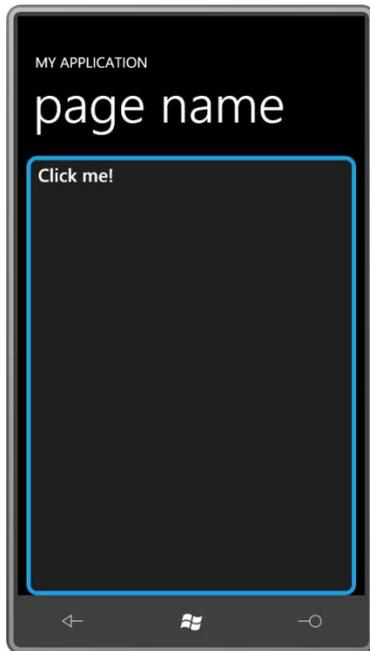
*Control* defines two properties named *HorizontalAlignment* and *VerticalContentAlignment* that are supposed to govern how the content is aligned within the *ContentControl*. If you set these properties on the button, you'll discover that they don't work.
