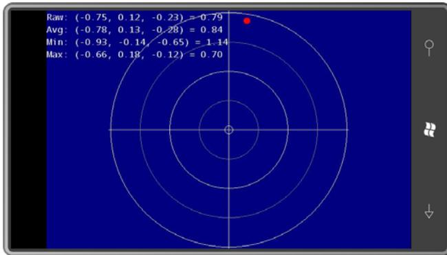
Increasing Y values of the accelerometer correspond with decreasing X values of the graphical display, and increasing X values of the accelerometer correspond with decreasing Y values of the graphical display. However, the intent here is to show a bubble that rises against gravity, so
