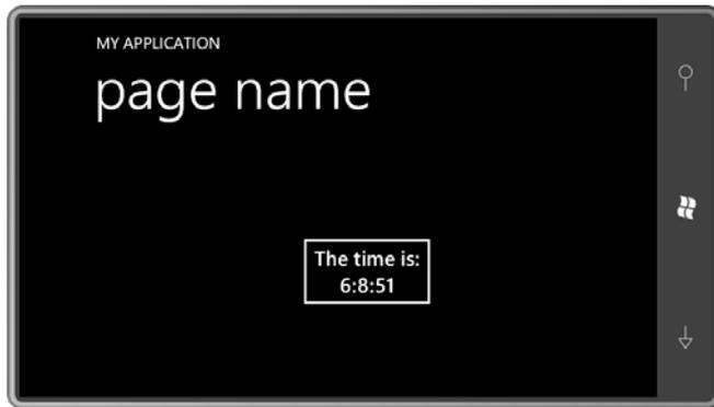
The displayed time is dynamically updated. Of course, the bindings for the *Minute* and *Second* properties should really reference a string-formatting converter to always be displayed with two digits.
