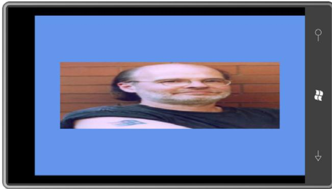
As you can see, there's nothing to prevent the image from losing its proper aspect ratio, as the calculations above imply. You can even—by sweeping your finger across the vertical center or horizontal center of the screen—cause the image to scale down to nothing!
