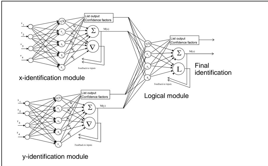
FIG. 5. Two recognition and one logical module of FSM.
