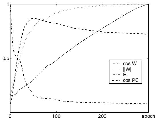
Figure 18: Change of parameters during network training. Vertical axis: normalized  $\|W\|$ , normalized MSE error,  $\cos(\mathbf{W}) = \cos(\mathbf{W}(t) - \mathbf{W}(t_{\max}))$ ,  $\cos(\mathbf{W}, \text{PCA}) = \cos$  between the weight vector  $\mathbf{W}$  and the resultant PCA direction. Horizontal axis shows epoch number  $t$ .
