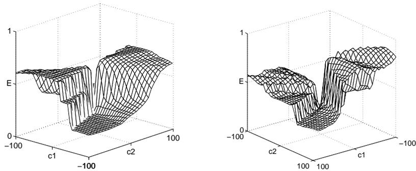
Figure 11: Left: ES of Ionosphere (42-4-2) with stretched sigmoid (stretch=1.3); right: ES of Iris (4-4-3) with staircase transfer function (5 stairs).
