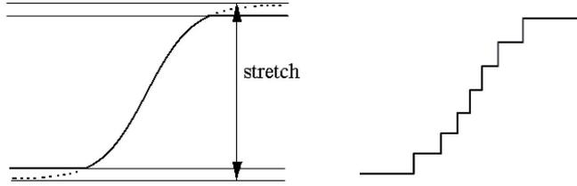
Figure 10: Transfer functions: a) stretched sigmoid, b) staircase function.
