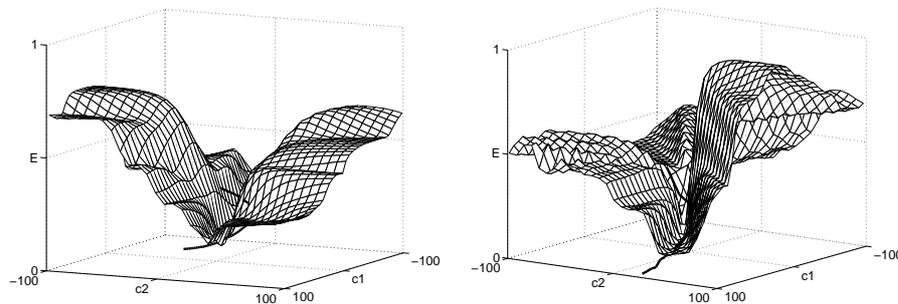
Figure 16: Left: ES and the learning trajectory of Iris (4-4-3) trained with backpropagation; right: trained with Levenberg-Marquardt algorithm.
